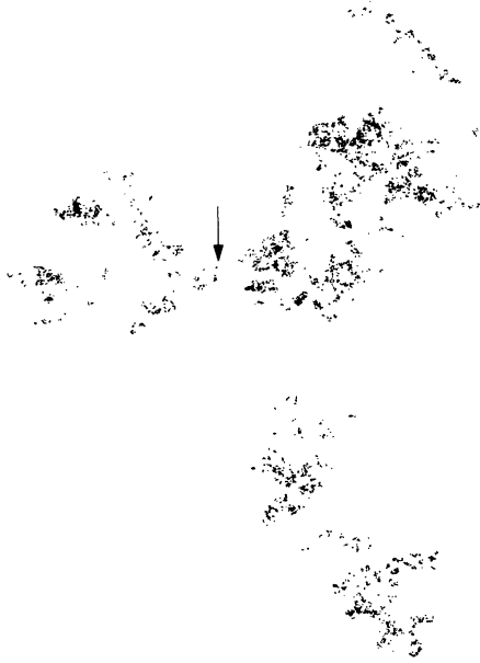
FIG. 1. The first 10^4 points visited by a random walker on the plane, with the jump probability density given in Eq. (8). The arrow indicates the initial position of the walker. The fractal dimension of this pattern is \gamma = 1.6 .
